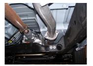
3. **2009/2010 Models Only** You will use part "I" to attach to the muffler re-using the factory clamp. Be sure that the tabs of the clamp are straight. If they are bent, it will not seal the connection
